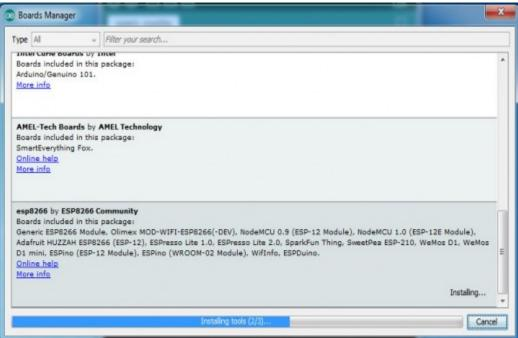
After installation, close the window and go to Tools> Board and see the list of available devices on the chip programming ESP8266
